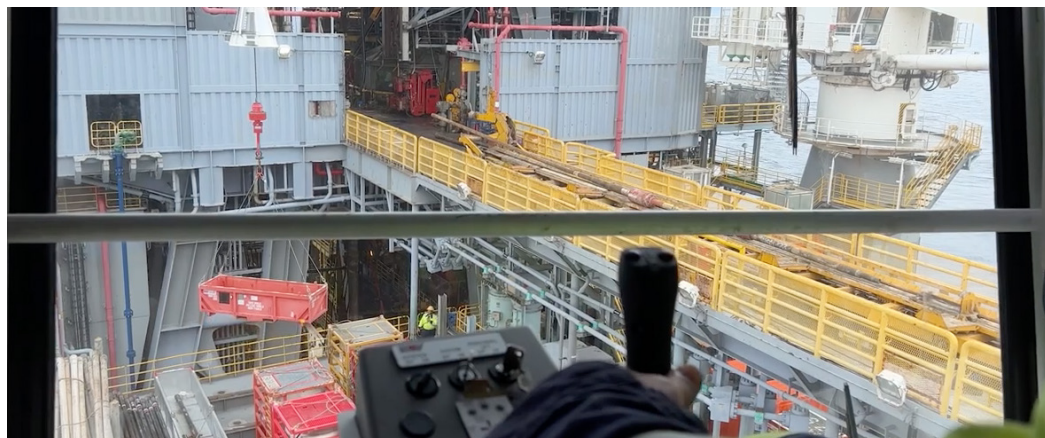
With the new crane technology, the crane operator can rotate the load 360 degrees while the deck crew stays safely out of range (Screenshot from Transocean's YouTube video about the technology).
