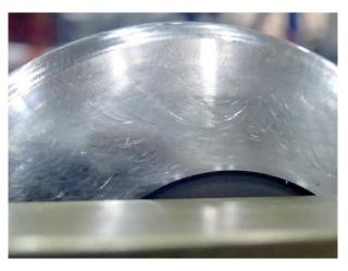
Arc-shaped scratches observed on the roller end of a worn axial tapered roller bearing from a top drive.
