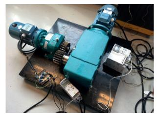
Figure 1: Laboratory setup with pitch drive (left) and load motor with bph gearbox (right)
