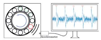
Figure 1: The bearing vibration is monitored using an accelerometer attached to the bearing housing.
