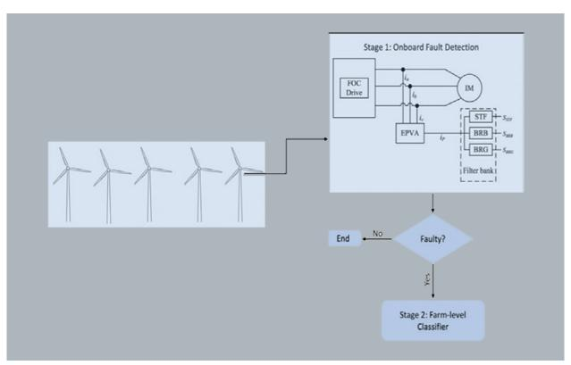
A two-stage fault detection and classification scheme for wind turbine pitch systems using AI.
