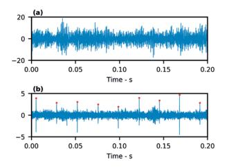
Figure 2: The raw vibration signal is filtered using an autoregressive model to highlight bearing faults. (a) The raw signal. (b) The filtered signal with red dots signalizing the bearing impact vibration.
