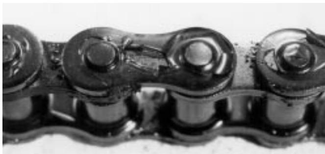
Paint-like residues on a test chain caused by high temperature
