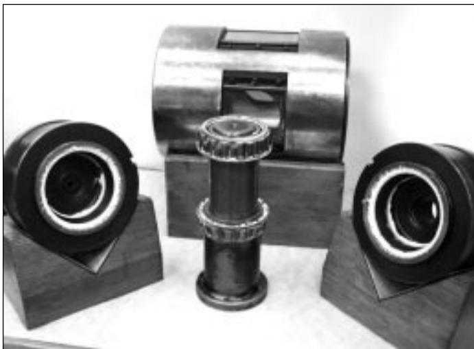
Shaft with disassembled test bearings, bushings and inspection glass
