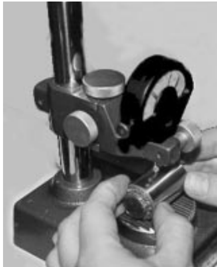
Measurement of bushing
