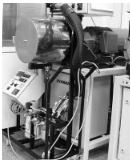
Test setup for oils, with thermal protection cover
