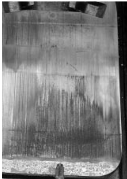
Wear pattern on switch plate
